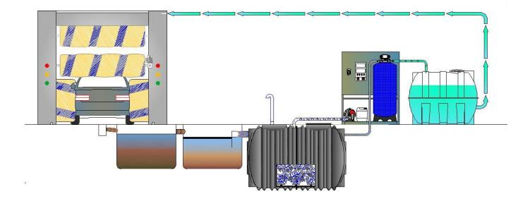
A complete line of carwash water treatment consists of a set of treatment operations, placed in series, with a view to achieving the predefined treatment objectives. In order to maximize water recovery and treatment, we recommend
